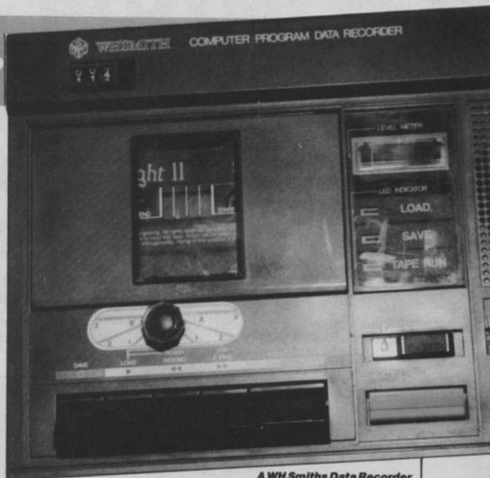
A WH Smiths Data Recorder with the LOAD IT azimuth adjuster
